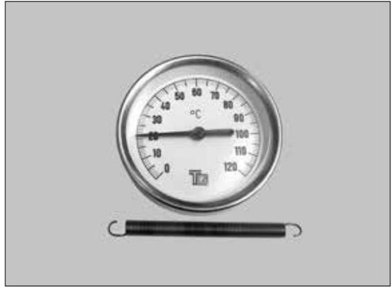
**Kode: P0340** Kontaktthermometer an Rohr
